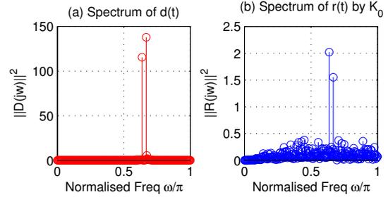
Fig. 4. (a) Disturbance Spectrum and (b) its frequency estimation through 512-point FFT-based residuals spectrum analysis
